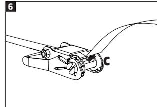
Thread the band through the slot in the axle ("C" in Image 6).
