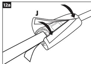
**IMPORTANT!** The slackline must not exceed two and a half rotations around the axle of the ratchet.
