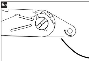
Additional information for the Surfer Line Ratchet and Andy Lewis Trickline: Please thread the slackline into the ratchet slot from the above when the ratchet facing upside down as indicated on the ratchet with an arrow. Please refer to Image 6a.
