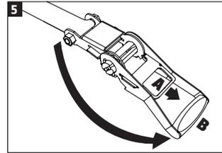
Release the ratchet (pull on the small lever inside the ratchet marked "A" in Image 5) and open the main lever ("B" in Image 5).
