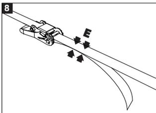
Once the band is taut through the axle, use one hand to hold both sides of the band together ("E" in Image 8 & 9).
